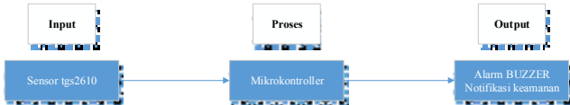
Gambar Error! No text of specified style in document.. Blok diagram sistem keamanan kebocoran gas LPG
